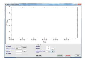
• CalSoft including for setting bath temperature and monitoring the PV. Graphical representations of PV/TIME with 2 hours data logging.
